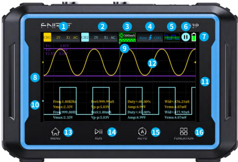
① **Channel 1 settings:** Channel on/off, vertical voltage, probe ratio, coupling type, and 20M bandwidth limit can be set.
