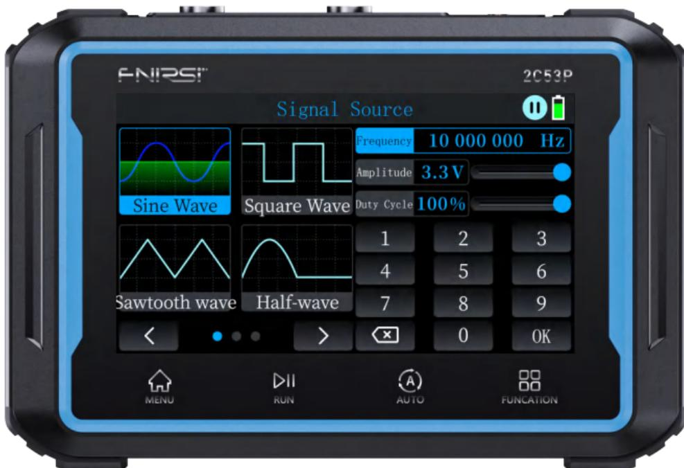
**① Signal type selection:** There are 12 types of waveforms to choose from, including sinusoidal wave, square wave, sawtooth wave, half wave, full wave, positive step wave, negative step wave, DC signal, exponential rise, exponential fall, multi-audio, and sync pulse.
